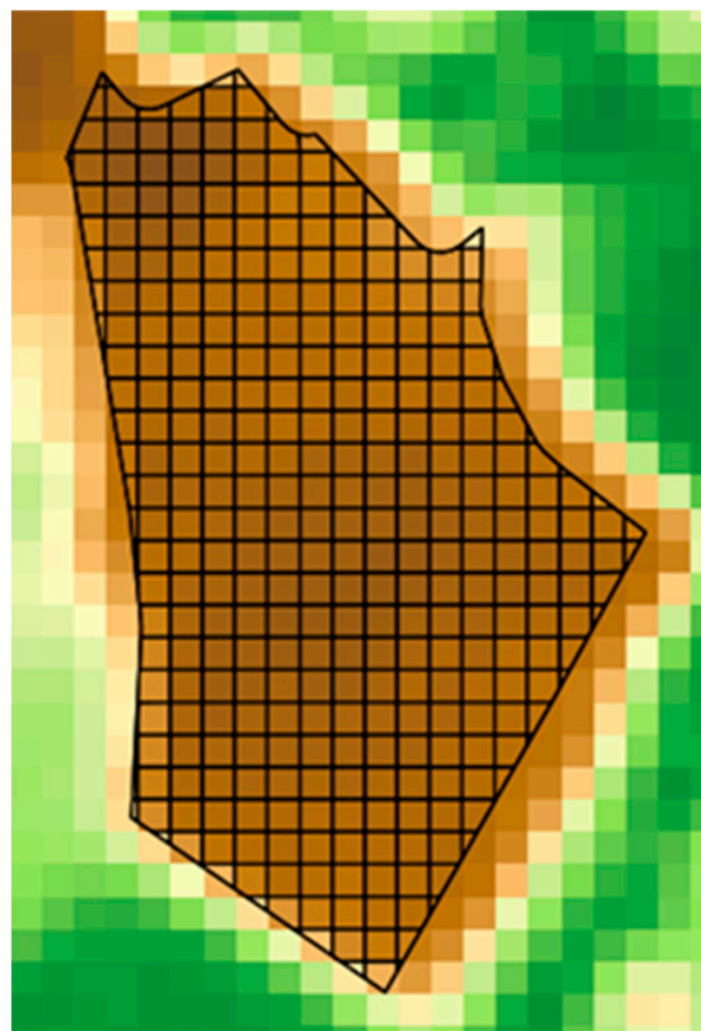
Figure 4. Extraction of pixel values contributing to the median satellite-derived biophysical variables at the field scale. Example of DMC-derived fAPAR after inward buffering.
