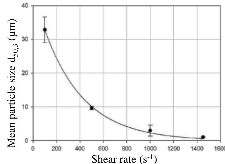
Influence of shear rate on the mean particle size  $d_{50,3}$  for a protein concentration of 30 wt % heated  $80^\circ\text{C}$  for 10 s with a degree of denaturation of > 95 %
