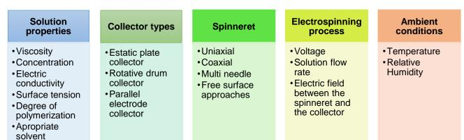
**Figure 2.** A summary of key parameters affecting the electrospinning process based on the knowledge described in the following references [25,28,37,39,47,52,53].
