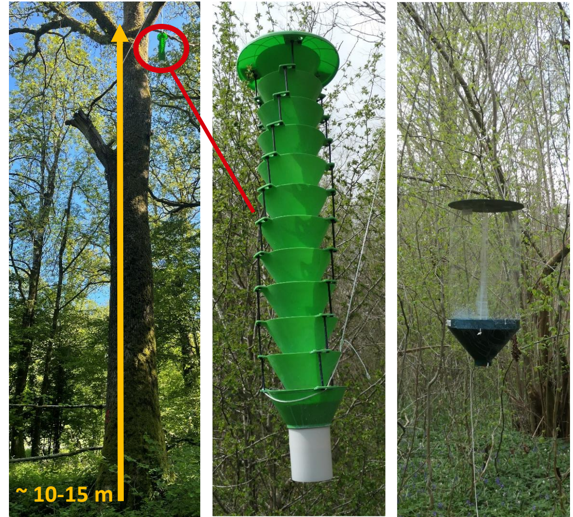
Oak canopy (left) with green multi-funnel trap (middle) & flight-interception trap (right). © E. Le Souchu
