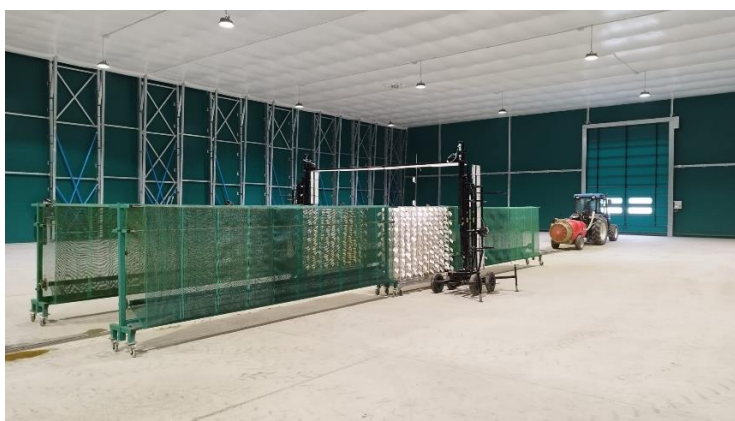
Fig. 1. General overview of experimental layout: artificial rows provided with small plastic collectors to mimic vine leaves and metal structure realised to surround the treated rows holding filter clothes collectors besides and over the applied rows.
