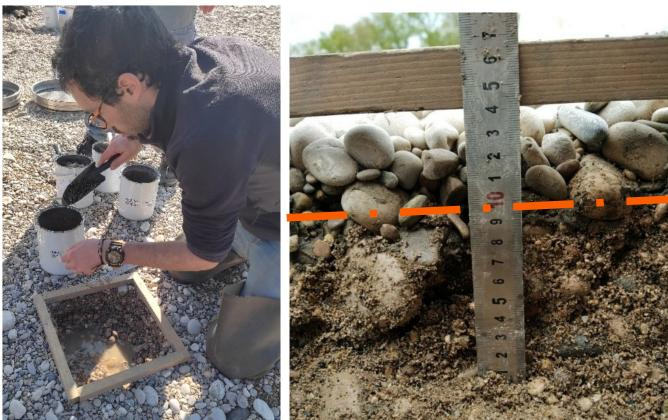
Sieving at 10mm, 2mm, 500µm and  $100\mu m$  with a volume V of water  $\rightarrow$  concentration C of sediments finer than 100µm
