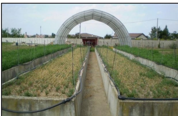
Figure 1. One of CRA-FLC's phenotyping platforms; it includes four environments formed by the combination of two soil types (sandy-loam or silty-clay) by two possible water regimes (applied via microirrigators under a moving shelter)
