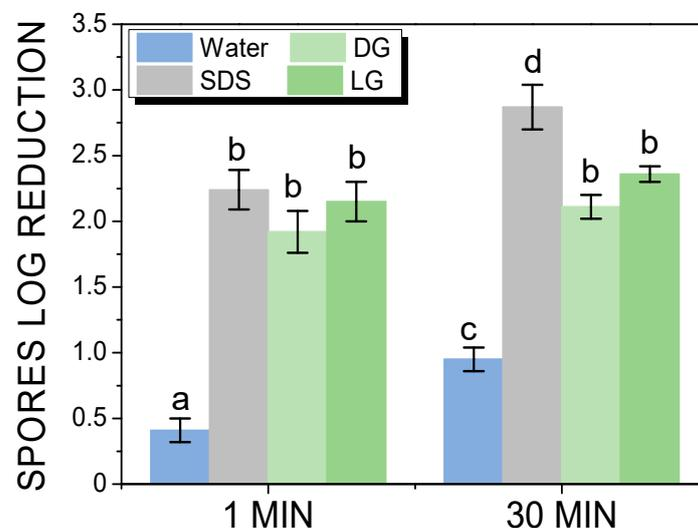
**Figure 2.** Spores log reduction on the plate in dynamic condition during foam flow cleaning after 1 and 30 min of foam flow as a function of the surfactant in comparison to water. The small letters a–d indicate groups of statistical differences according to Tukey's test ( $p < 0.05$ ) between the water and the surfactants for 1 min of foam flow cleaning and for 30 min of foam flow cleaning.
