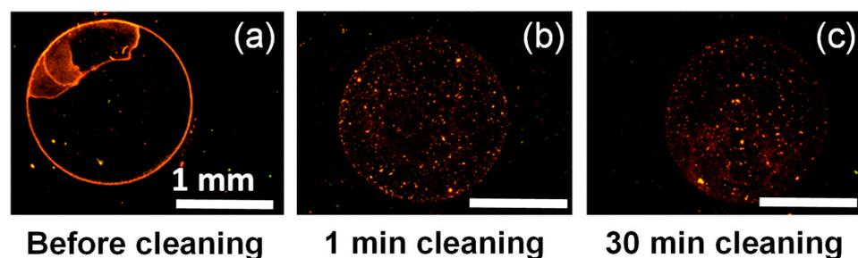
**Figure 3.** Epifluorescence microscopy pictures of a stainless-steel plate contaminated by spores and stained with acridine orange: (a) before cleaning by foam flow, (b) after one minute of foam flow cleaning based on DG, and (c) after 30 min of foam flow cleaning based on DG. The scale bar represents 1 mm for all the pictures.
