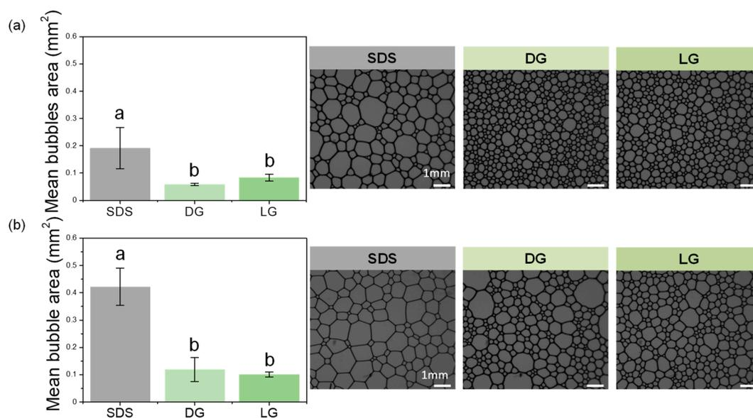
**Figure 5.** Mean bubbles area of the foams produced with SDS, DG, and LG with the corresponding microscopic pictures: (a) before the foam passed through the duct containing the plate contaminated with spores and (b) after the foam passed through the duct. The scale bar represents 1 mm for all the foam pictures. The small letters a–b indicate groups of statistical differences according to Tukey’s test ( $p < 0.05$ ).
