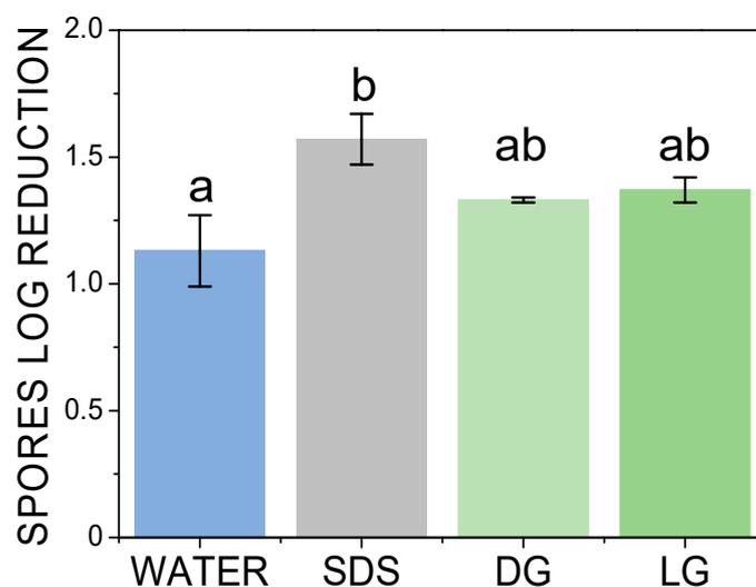
**Figure 1.** Spores log reduction on the plate under static dipping conditions as a function of the surfactant in comparison to water. The small letters a–b indicate groups of statistical differences according to Tukey's test ( $p < 0.05$ ).
