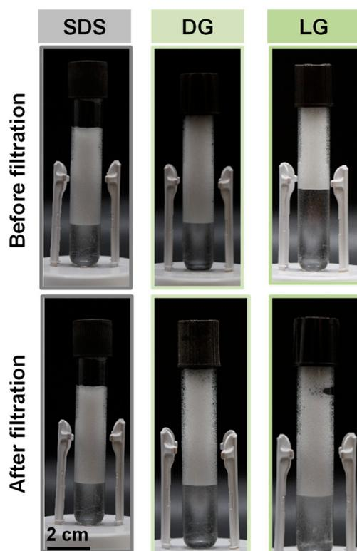
**Figure 6.** Pictures of the foams produced from the surfactants solution (SDS, DG, and LG) before and after filtration to remove the spores, showing a similar foamability and foam stability around 5 min after producing the foam. The scale bar represents 2 cm for all the pictures.
