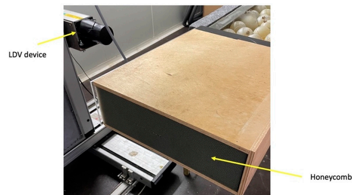
Figure 3. Image of the LDV measuring device and the honeycomb at the inlet of the tunnel.
