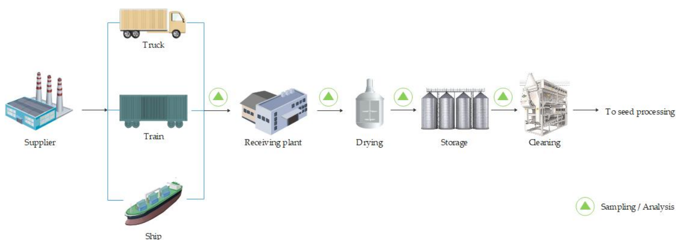
Figure 1. Typical processes in the reception and storage of oilseeds.
