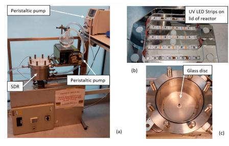
**Figure 2.** (a) SDR. A peristaltic pump circulates the water around the vessel and cooling water around the water jacket. (b) UV LED strips attached to the bottom of the lid of the reactor. (c) Image of the internal view of the SDR with a  $TiO_2$ -coated disk held in place by the central metal rod.
