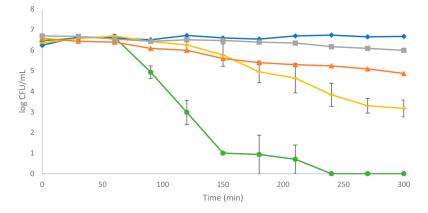
**Figure 5.** Photocatalytic inactivation of *E. coli* in the SDR using borosilicate disks coated with either a ZnO or TiO<sub>2</sub> film with the addition of PEG to aid bonding: (blue  $\blacklozenge$ ) dark control; (gray  $\blacksquare$ ) ZnO dark control; (orange  $\blacktriangle$ ) light control; (yellow —) photocatalysis with a TiO<sub>2</sub> disk; (green  $\blacklozenge$ ) photocatalysis with a ZnO disk. Three replicate experiments were performed.
