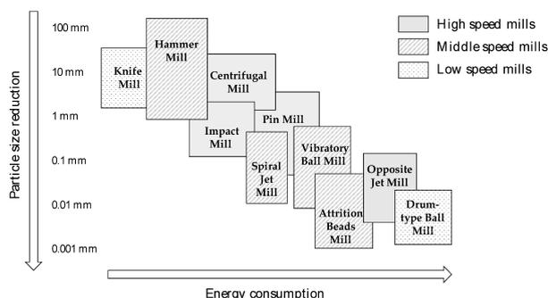
Figure 1. Exemplification of how the energy consumption increases in relation to the particle size reduction (Mayer-Laigle C., Rajaonarivony, R., *et al*, 2018).
