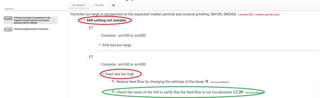
Figure 14. Example of the decision tree “Particles too large in comparison to the expected median particle size {coarse grinding, SM100, SM300}”
