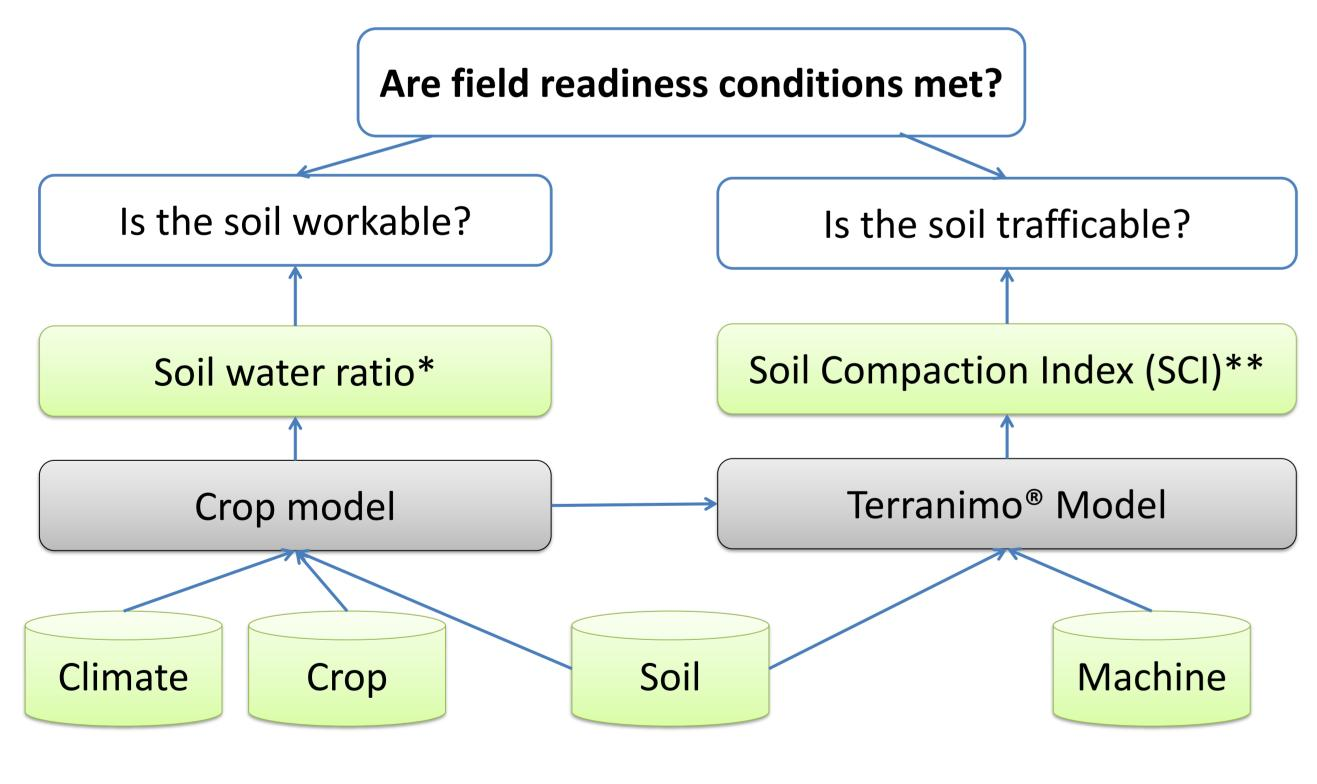
Figure 1 : Functioning of J-DISTAS tool to determine soil readiness. \*Soil water ratio is defined in part 3.2 materials and methods \*\* SCI = log(Pact/Pc) with Pact = vertical stress, Pc= soil strength (Schjønning and Lamandé, 2020)
