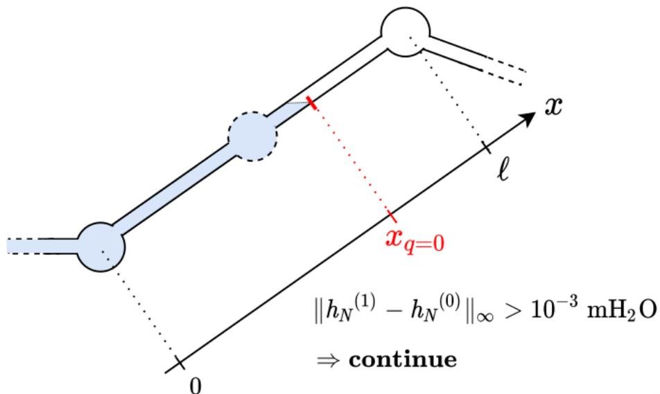
Steps 3, 4, 5, ...: **repeat** the same process as at step 2, until convergence of the discretization algorithm.
