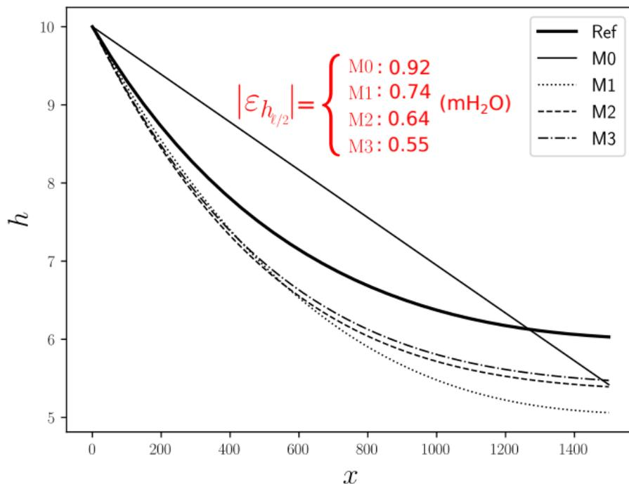
$\Rightarrow$  models  $\{M1, M2, M3\}$  compute **better predictions** of heads than M0, especially at **intermediate positions**
