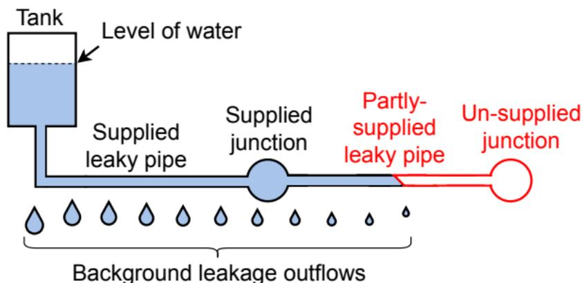
⇒ neglecting them can lead to **miscomputation** of the hydraulic grade lines (**HGLs**).
