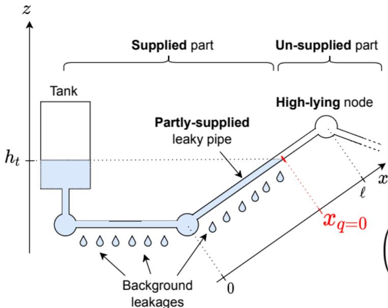
... then, in each pipe where  $x_{q=0}$  exists, use it to **correct** the flow rates at pipe's extremities:
