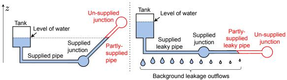
$\Rightarrow$  neglecting them can lead to **miscomputation** of the hydraulic grade lines (HGLs).
