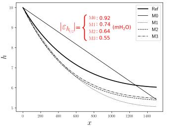
$\Rightarrow$  models  $\{M1, M2, M3\}$  compute better predictions of heads than M0, especially at intermediate positions
