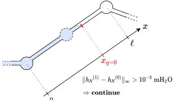
Steps 3, 4, 5, ...: **repeat** the same process as at step 2, until convergence of the discretization algorithm.
