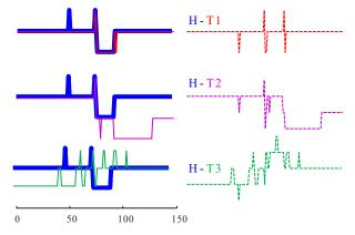
Figure 6: *left*) The hypotheses overlaid with three candidate time series. *right*) Subtracting the time series from the hypotheses produces a *difference vector*, the "simplicity" of which is suggestive of similarity of the two signals.
