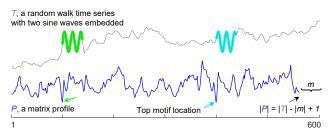
Figure 3: A synthetic time series T which has two (highlighted) motifs imbedded, and its matrix profile P. Note that P minimizes at the location of the motifs.
