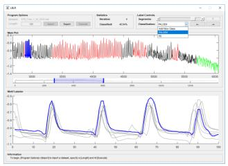
Figure 19: A snapshot of our deployed implementation of LBLR. After performing four iterations, the user is in the process of brushing the phloem label onto the subsequences identified in the bottom cluster. These changes will be reflected in the top graph and the user will again be shown another candidate cluster of subsequences.
