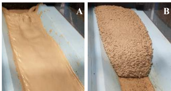
Fig. 3. Calibration flume tests: propagation of A: fluid mixture, B: viscous mixture
