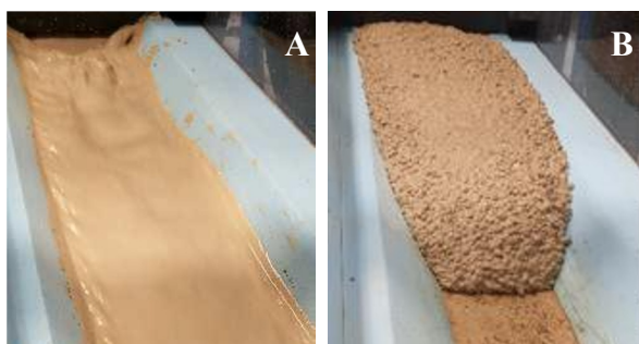
Fig. 3. Calibration flume tests: propagation of A: fluid mixture, B: viscous mixture
