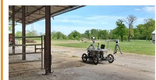
It verifies the accuracy of execution of a proposed path in a «farmyard» environment, incorporating different types of perturbations
