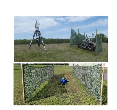
ARPA PC1 evaluates execution accuracy of robots trajectories in field production
