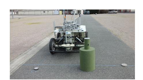
The test assesses the robot's ability to detect and stop when it encounters a reference obstacle in its detection zone
