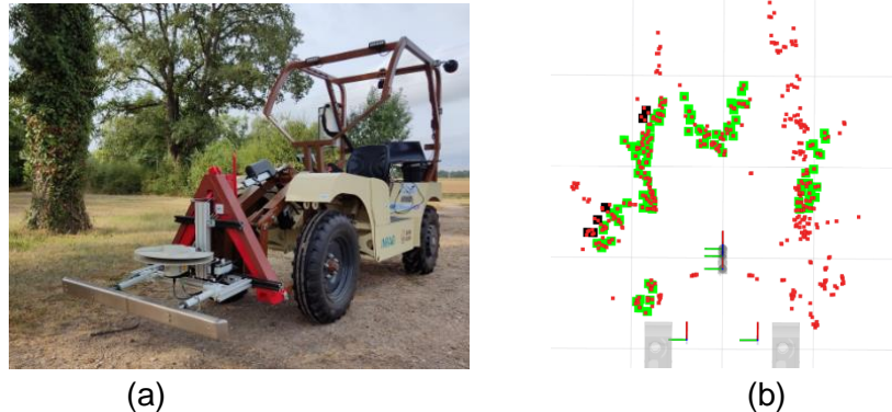
Figure 13. (a) ALPO tractor robot equipped with SBPS and LMS Sick LiDAR, (b) Classification using LiDAR in tall grass field (green=traversable obstacles, black= non-traversable obstacles and red=non-identified obstacles)
