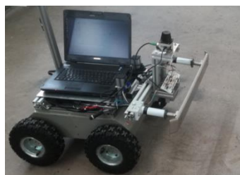
Figure 6. Sensitive bumper probing system mounted on "Effibote3 Robot"
