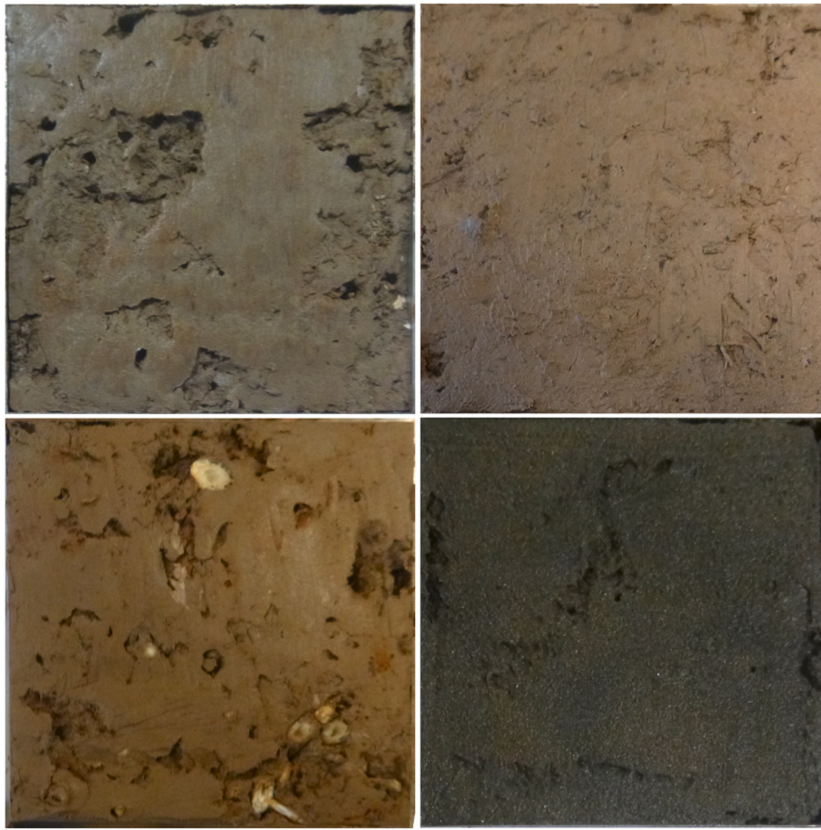
Fig. 3. Vertical photographs of Shear box samples from four surface cover types. Top left TF BARE, top right TF PUC, bottom left TF SPA, bottom right WS BARE. Samples are 60 × 60 mm and are sheared along the plane depicted.
