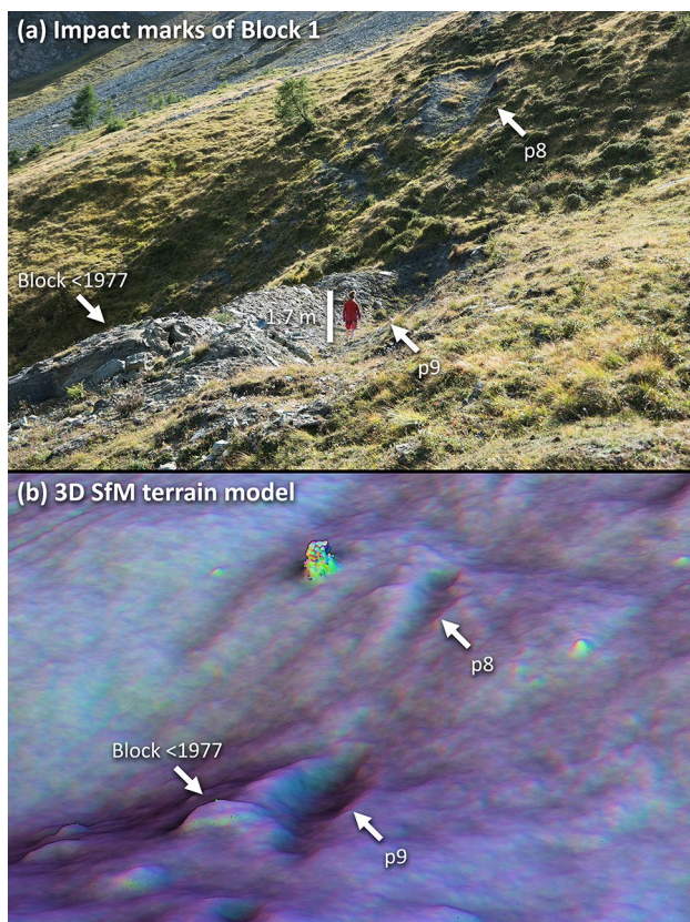
Fig. 8 Two impact marks from block 1, numbered p8 and p9, visible on a photo taken in September 2019 in (a) and on the artificially colored 3D SfM terrain model in (b). A block fragment from a previous rockfall event that occurred before 1977 based on the oldest orthophoto covering the site lies next to impact mark p9
