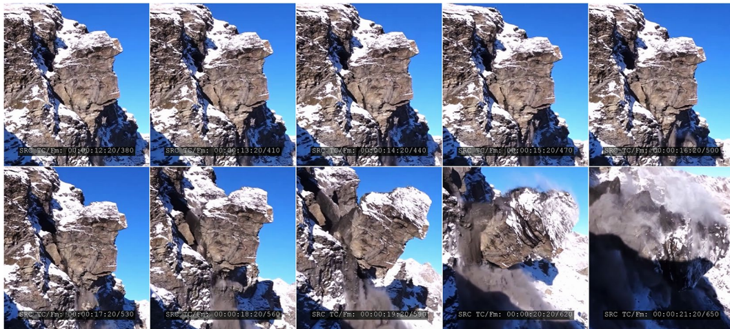
Fig. 4 Selected frames seconds apart of the video footage captured near the source cliff showing the toppling failure of the 2015 rockfall event. The cropped part of the video has a field of view (FOV) of approximately 65°
