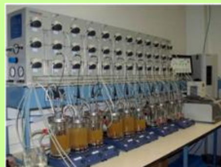
Simulator of the Human Intestinal Microbial Ecosystem (SHIME)
