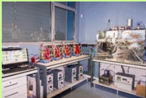
SIMulator of the GastroIntestinal tract (SIMGI)
