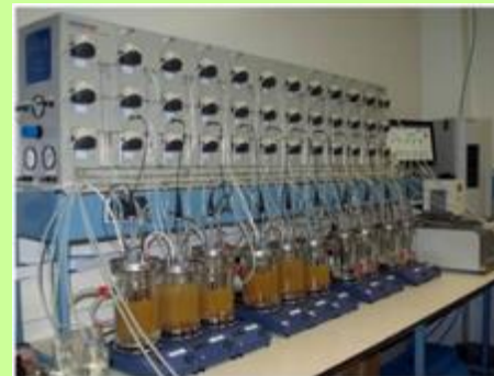
Simulator of the Human Intestinal Microbial Ecosystem (SHIME)
