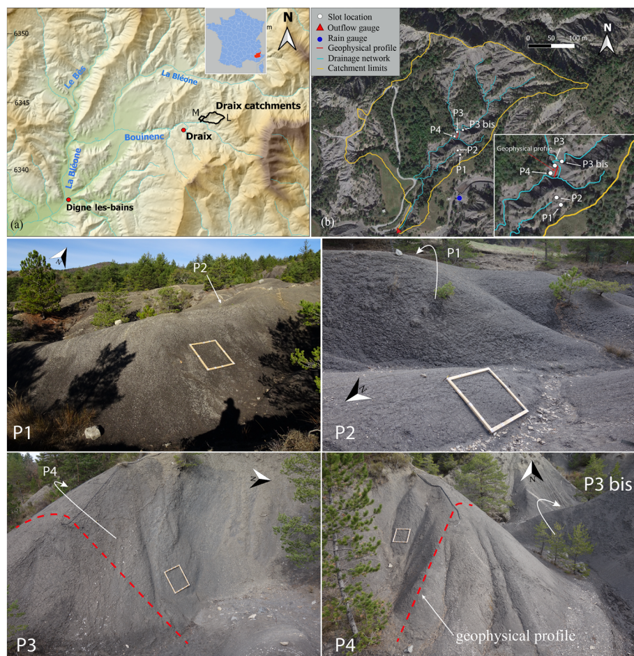
FIGURE 1 Geographic setting of the Draix–Bléone Critical Zone Observatory and of the measurement sites. (A) Shaded relief map (from the DEM RGEALTI IGN database) of the Bouinenc drainage basin and location of the monitored catchments (black outlines; L: Laval; M: Moulin). Inset shows location in France. (B) Satellite image (Google Earth) of the Moulin catchment. Inset shows a zoom on the measurement plots and the location of the geophysical profile. Lower images (P1–P4) are field photographs of the different measurement plots (wooden frame is 1 × 1 m); east facing and parallel to the schistosity (P1); west facing and perpendicular to the schistosity (P2); north-facing (P3); and south facing (P4). Red dashed line shows the location of the geophysical profile [Color figure can be viewed at wileyonlinelibrary.com ]
