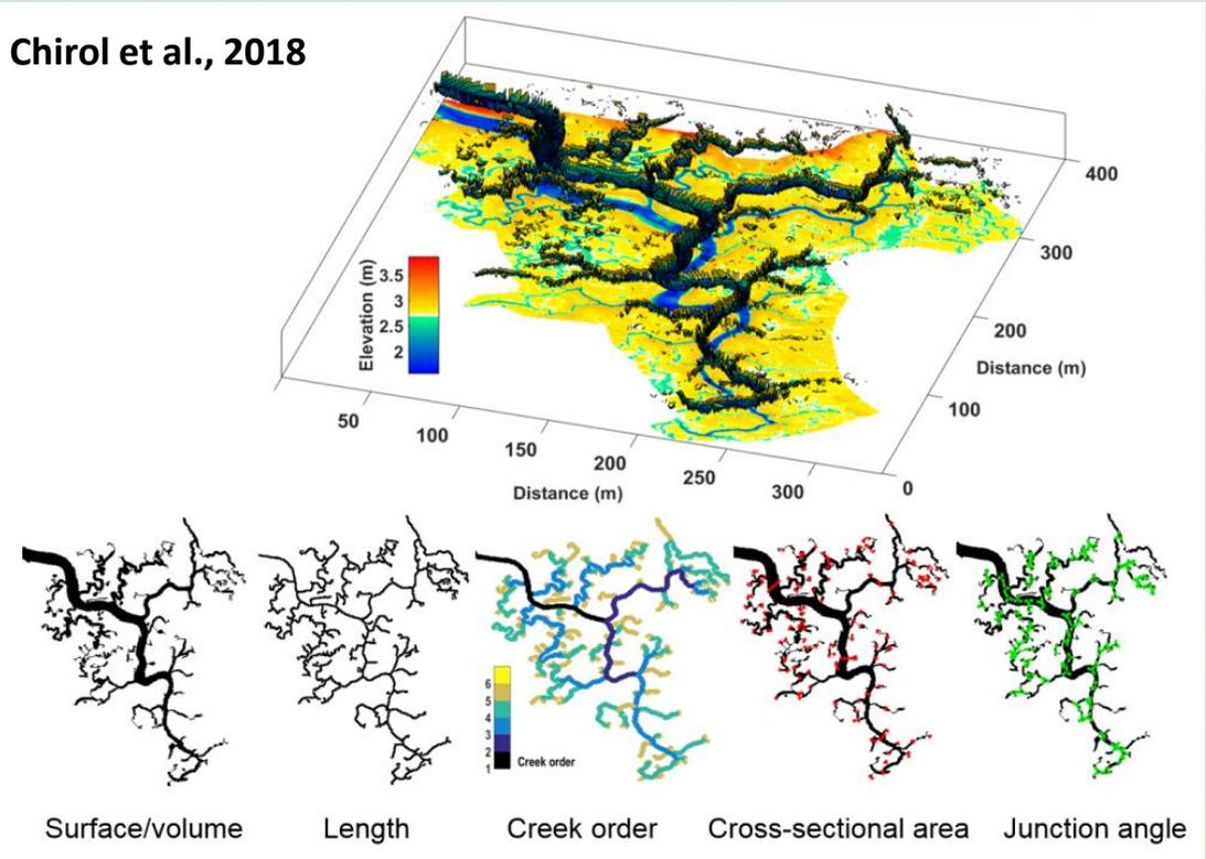
Semi-automated algorithm developed to extract key shape parameters of saltmarsh creeks
