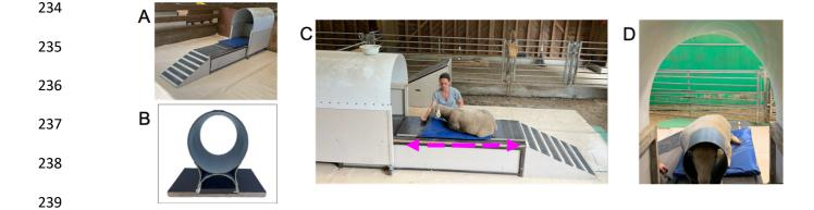
Learning MRI Acquisition Related Behaviors. A) The mock MRI scanner composed of a ramp, a fixed base on which a mock patient bed sits and a mock bore; B) The mock RF head coil; C) Ted lying down on the moveable mock MRI table (dashed pink arrow), on a comfortable blue mat, in front of the mock MRI bore; D) Léonard waiting motionless with his head inside the mock RF head coil.
