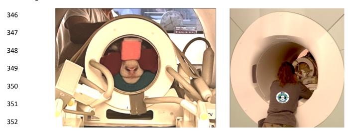
353 Sheep performing brain MRI acquisition. A) The head position in the sheep RF coil. The head is 354 "blocked" with foam pieces adapted to each individual. A trainer is at the front of the bore with a hand 355 placed on the sheep's back; B) The other trainer sat at the back of the bore, facing the sheep, to 356 maintain visual contact.
