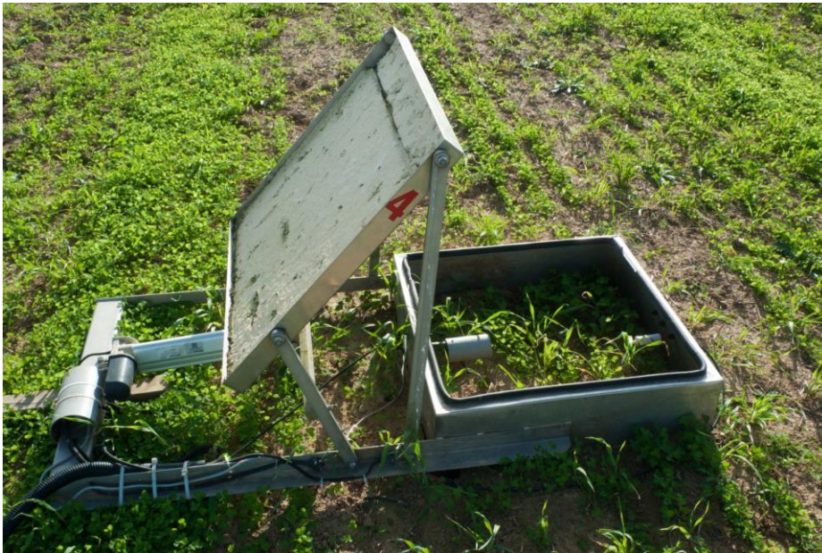
Automatic chamber monitoring N 2 O fluxes
