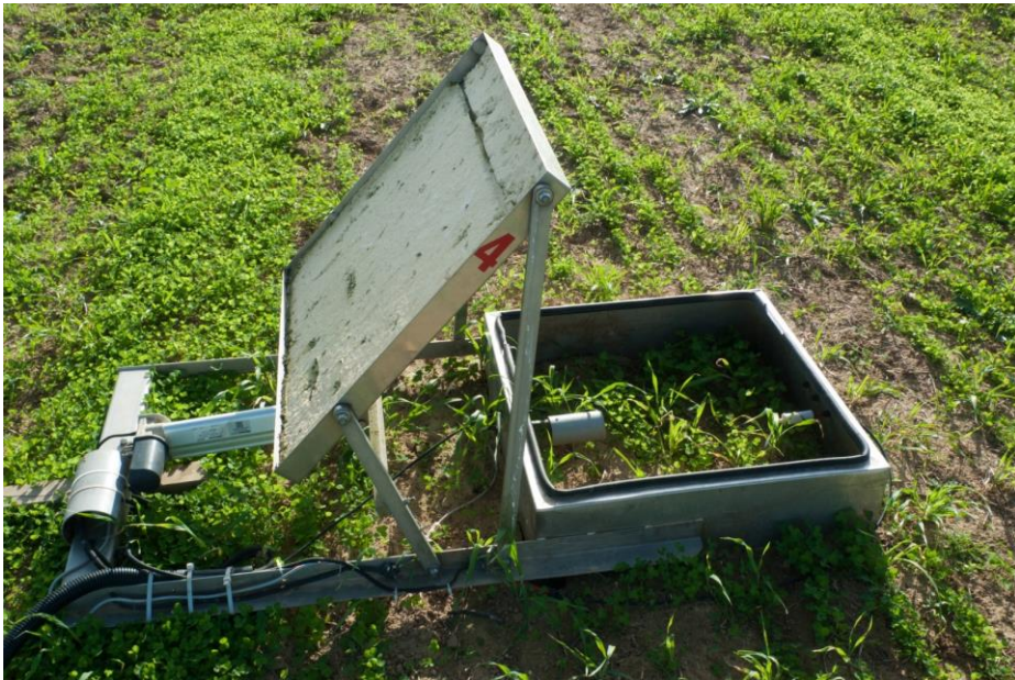
Automatic chamber monitoring N 2 O fluxes
