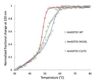
**Fig. 3.** Temperature denaturation of wild-type and variants AmGSTD1 followed by the normalized fractional change at 220 nm measured from CD experiments. The data were fitted with the CDPAL software and each experiment was performed in triplicate.
