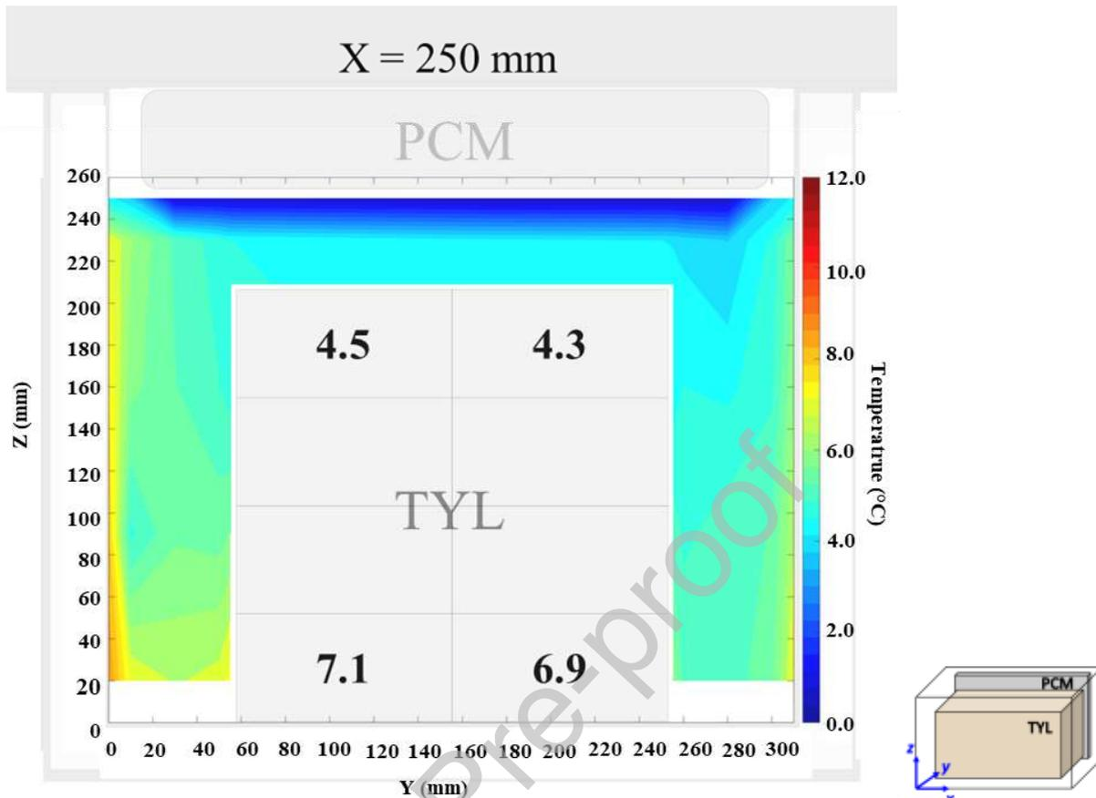
Figure 12: Air temperature field and core temperature of test product ( $^{\circ}\text{C}$ ) on the middle plane in a loaded horizontal box with PCM at the top under  $20^{\circ}\text{C}$  ambient, product initial temperature =  $4^{\circ}\text{C}$  without gap below
