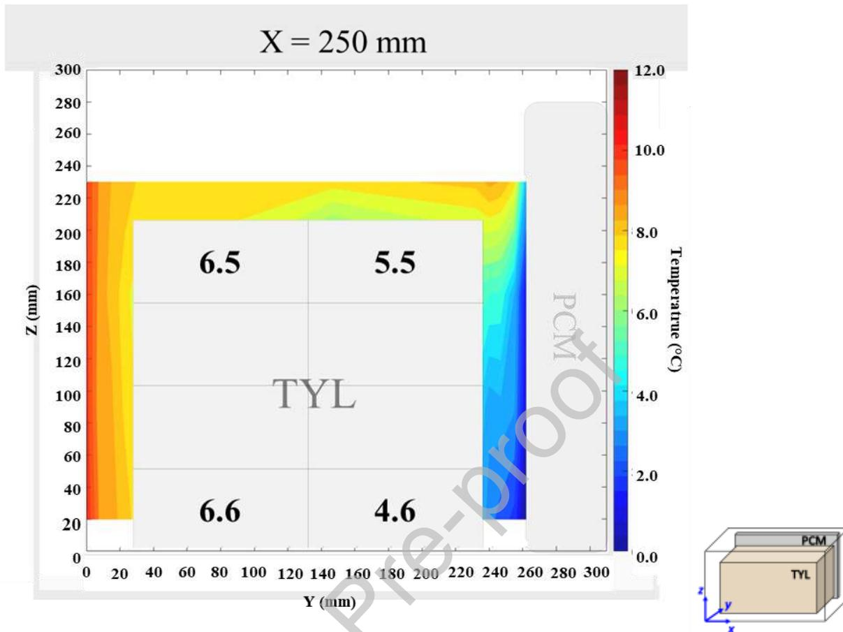
Figure 11: Air temperature field and core temperature of test product ( $^{\circ}\text{C}$ ) on the middle plane in a loaded horizontal box with PCM on a sidewall under  $20^{\circ}\text{C}$  ambient, product initial temperature =  $4^{\circ}\text{C}$  without gap below
