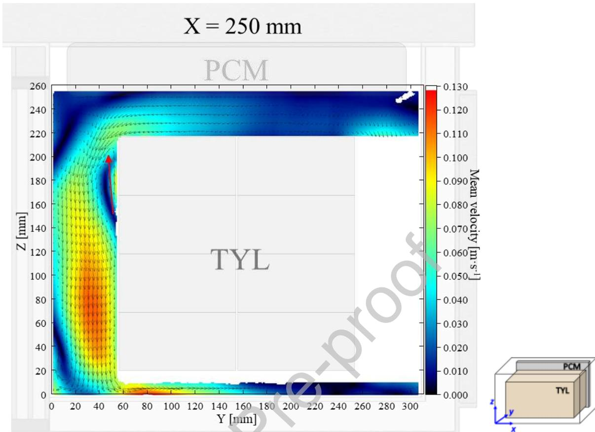
Figure 7: Air velocity field on the middle plane in a loaded horizontal box with PCM at the top under 30°C ambient, product initial temperature = 4°C with 20 mm gap below. White area on the right represents the unmeasurable zone because of the inaccessibility of laser sheet.
