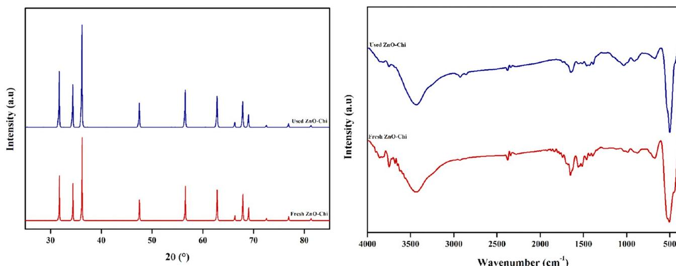
Figure 11. XRD and FTIR of ZnO-Chi before and after photocatalytic degradation.
