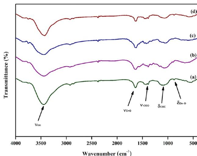
**Figure 2.** FTIR spectra of xerogels: Zn@Alg-X (a), Zn@Chi-X (b), Zn@CMC-X (c), and Zn@Pec-X (d).
