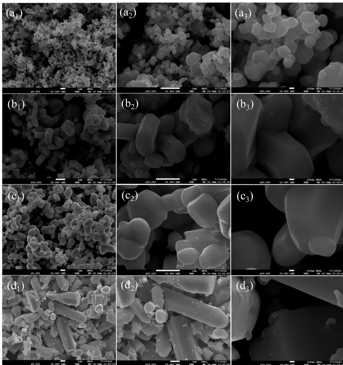
**Figure 6.** FEG-SEM images of the ZnO NPs that form during the calcination of the prepared xerogels via biopolymer gelation: ZnO-Alg (a<sub>1</sub>, a<sub>2</sub>, a<sub>3</sub>), ZnO-Chi (b<sub>1</sub>, b<sub>2</sub>, b<sub>3</sub>), ZnO-CMC (c<sub>1</sub>, c<sub>2</sub>, c<sub>3</sub>), and ZnO-Pec (d<sub>1</sub>, d<sub>2</sub>, d<sub>3</sub>).
