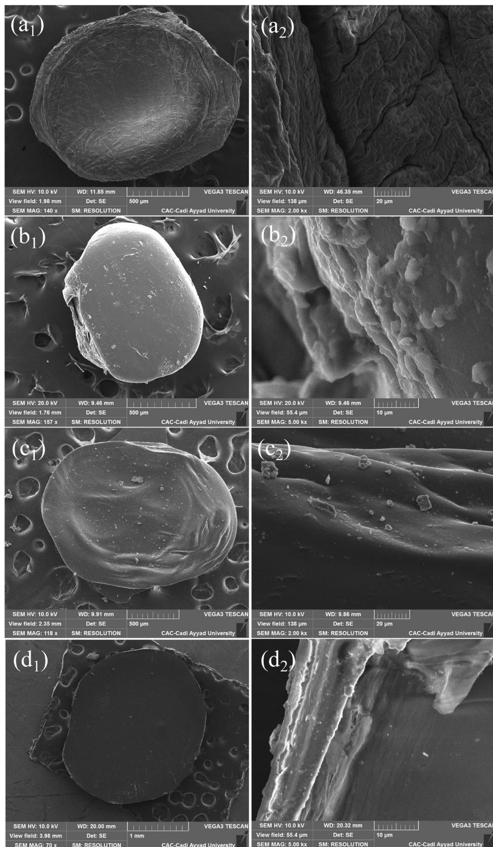
**Figure 3.** FEG-SEM images of Zn@Alg-X (a<sub>1</sub>, a<sub>2</sub>), Zn@Chi-X (b<sub>1</sub>, b<sub>2</sub>), Zn@CMC-X (c<sub>1</sub>, c<sub>2</sub>), and Zn@Pec-X (d<sub>1</sub>, d<sub>2</sub>).
