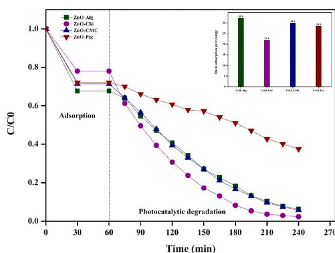
**Figure 8.** Adsorption–photocatalytic degradation activity of as-prepared ZnO nanoparticles.
