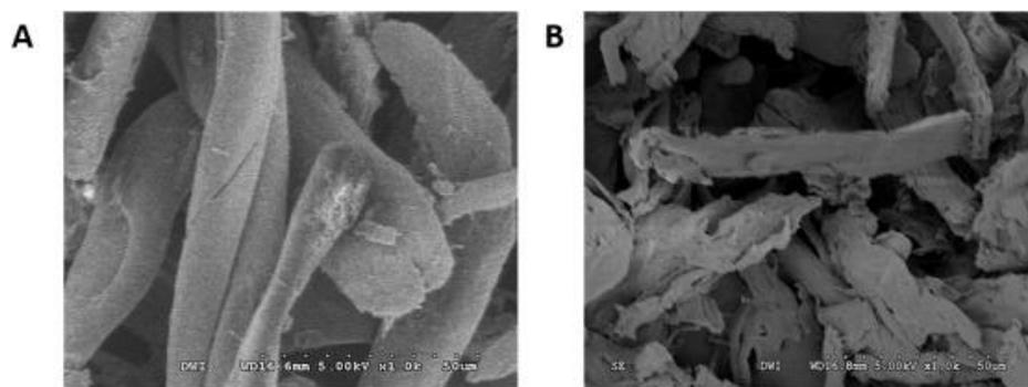
**Fig. 2.** SEM micrographs of (A) AVICEL cellulose ( $\times 1000$  magnification) and (B) *Ulva lactuca* cellulose ( $\times 1000$  magnification).
