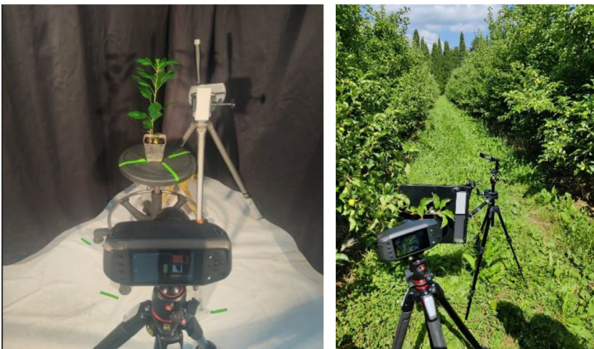
Fig. 5. Hyperspectral image acquisition setup. On the left, in laboratory conditions, and on the right, in the orchard.
