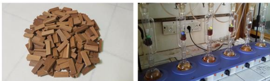
Fig 1: (a) Sanded specimens 30×10×5 mm 3 ; (b) Extraction of the test pieces using Soxhlet.
