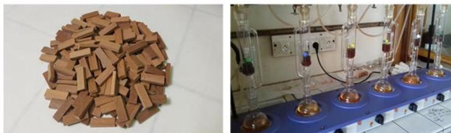
Fig 1: (a) Sanded specimens 30×10×5 mm<sup>3</sup>; (b) Extraction of the test pieces using Soxhlet.
