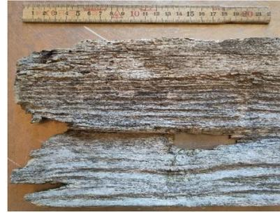
Fig. 2 : A "tavillon" of Alder from the façade on Fig. 1 is showing a nail hole, which has become bigger and where crack formed from it to the edge.
