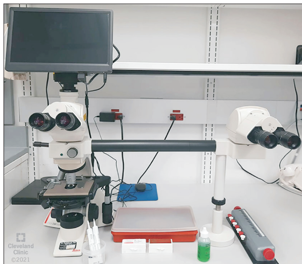
Fig. 3. Phase contrast microscope station for evaluating the presence of antisperm antibodies (ASA).
