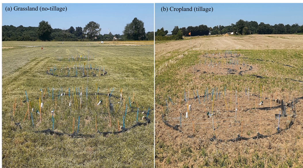
Fig. 1. In-situ whole-soil warming experiment under contrasting grassland management: (a) continuous grassland; and (b) cropland (cropland phase after 6 years of ley grassland) in a temperate region of western France.
