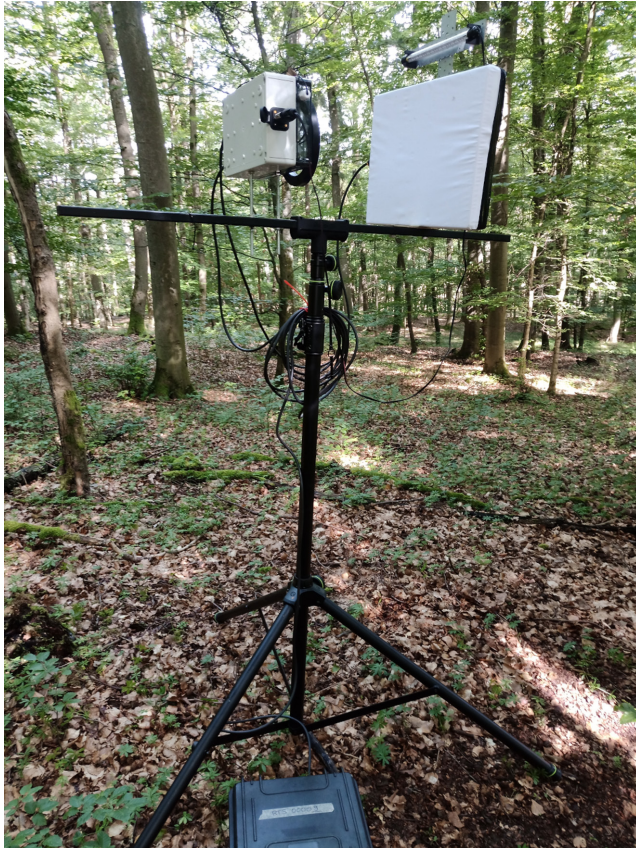
FIGURE 9 Insect monitoring. Automated moth trap for monitoring insect abundance by capturing photos of attracted moths via UV-light. Photo: L. Heidrich.
