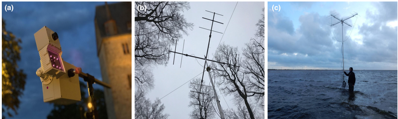
FIGURE 2 BatRack . BatRack is a multi-sensor monitoring solution that combines individual methods for the monitoring of bats, consisting of automatic VHF radio tracking, as well as audio and video recording combined in a single platform (a). Each sensor can be used as a trigger for the other, thereby strongly improving detection rates. BatRack allows researchers to efficiently collect data on species occurrences at a very high spatiotemporal resolution and can reliably operate in various environments (a–c). Photos: P. Lampe (a), J. Gottwald (b), V. Salewski (c).
