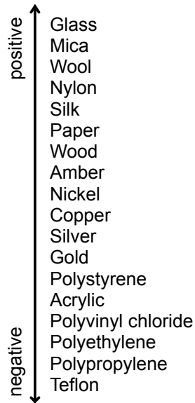
Figure 4: Typical example of triboelectric series adapted from [44].
