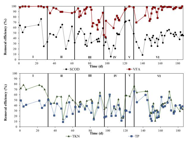
**Figure 1**. Removal efficiencies of (up) SCOD and VFAs and (down) total Kjeldahl nitrogen (TKN) and total phosphorus (TP) at the different operation periods. The roman numbers refer to the phases described in Table 1. Adapted from Hülsen et al. (2022b).
