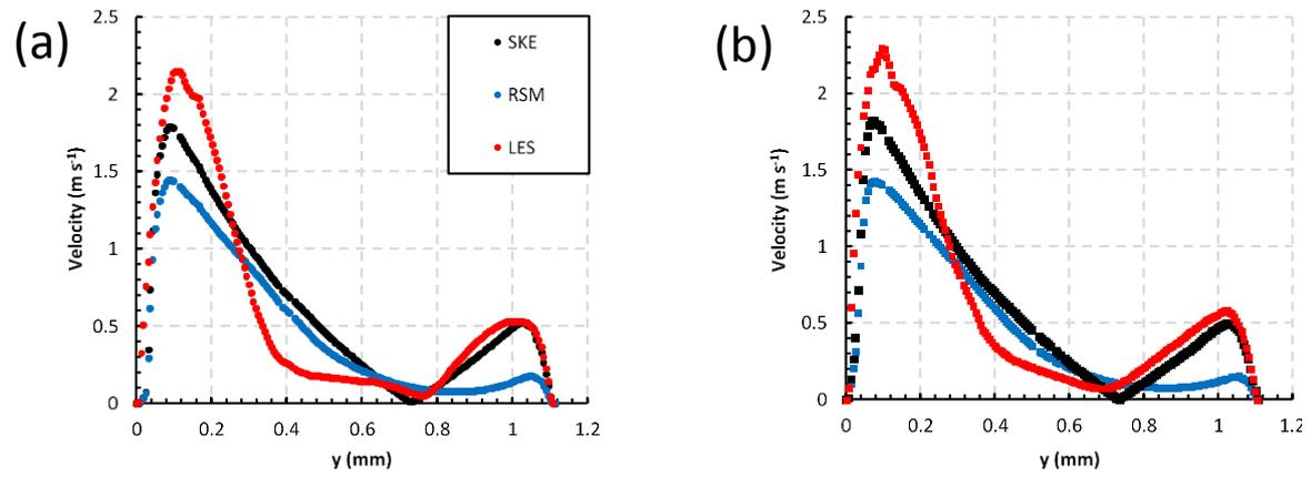
**Fig. 7.** (a) comparison of the velocity profile at baffle number 6 (I4), (b) comparison of the velocity profile at baffle number 25 (I8).
