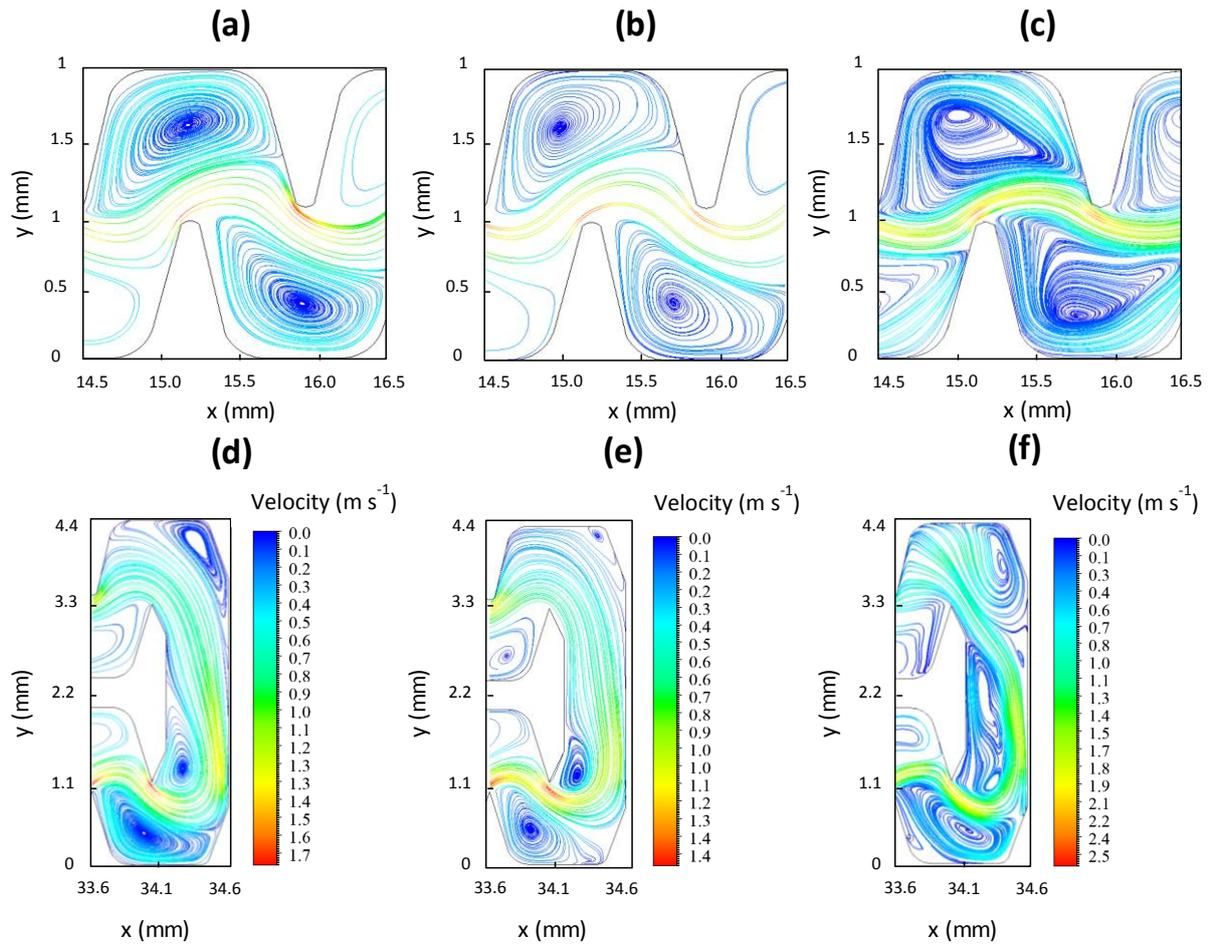
**Fig. 5.** Velocity streamlines at the inlet zone (a, b, and c for the SKE, RSM, and LES models, respectively) and at the return (d (SKE), e (RSM), and f (LES)) zone. Results are presented at  $z = 0.4$  mm.
