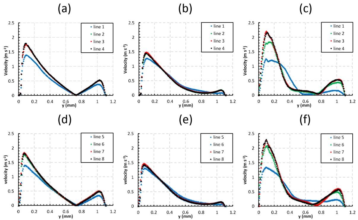
**Fig. 6.** Velocity profiles of different turbulence models at key sections of the emitter: SKE (a), RSM (b), and LES (c) at the first baffles in the inlet zone and at the first baffles after the return zone (d (SKE), e (RSM), and f (LES)). The order of lines 1 to 8 corresponds to the baffle numbers 1, 3, 4, 6, 20, 22, 23, and 25 respectively. All lines are plotted in Fig. 1.
