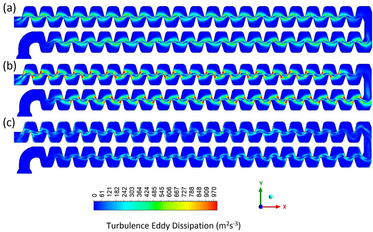
**Fig. S2.** Turbulence eddy dissipation obtained at  $z = 0.4$  mm using SKE (a), RSM (b), and LES (c) models.
