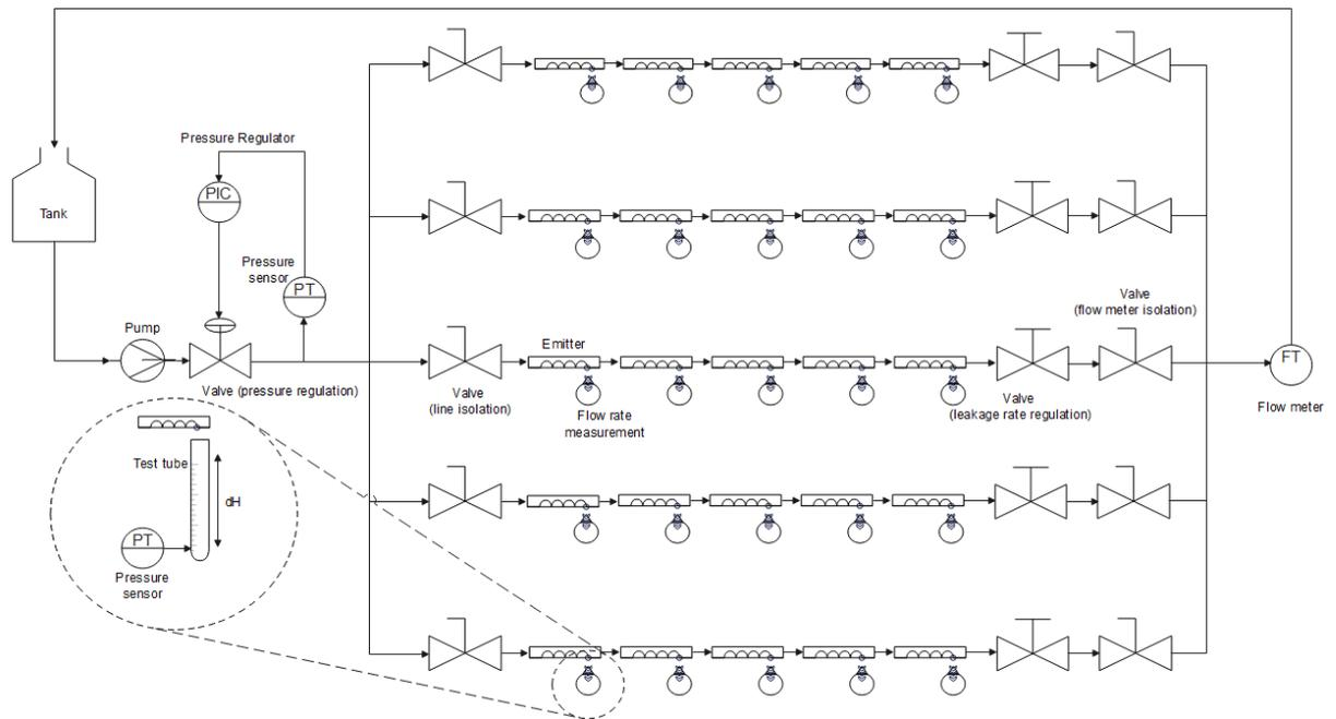
**Fig. 2.** Schematic representation of a pilot rig illustrates emitter discharge **was evaluated** by measuring flow rates and pressure losses in 25 emitters across 5 parallel lines.
