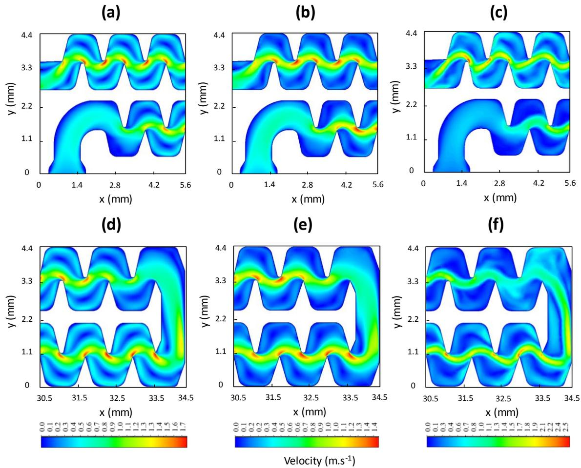
**Fig. S1.** Representation of the mean velocity fields at the selected area of the labyrinth (black rectangles): the inlet (a, b, and c for the SKE, RSM, and LES models, respectively) and the return (d (SKE), e (RSM), and f (LES)). Results are presented at  $z = 0.4$  mm.
