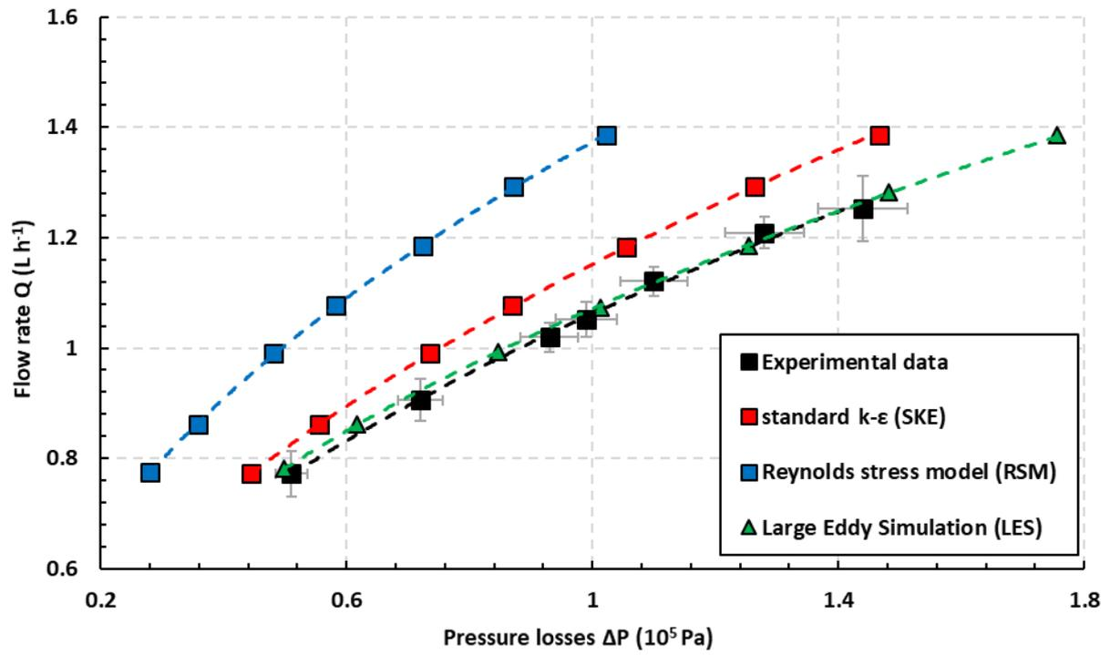
**Fig 3.** Discharge-pressure loss curves for the different turbulence models (CFD) and experimental data.
