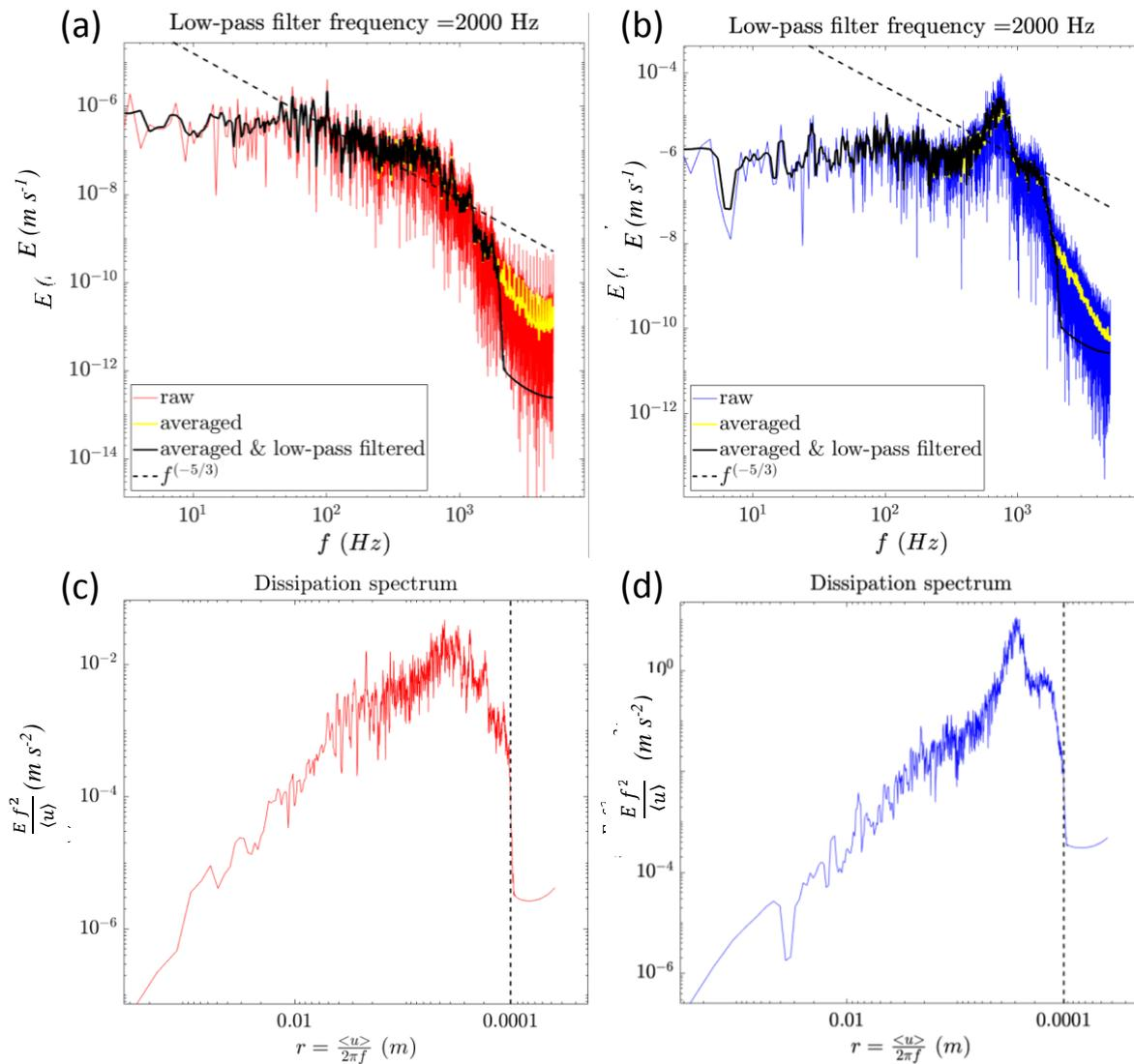
**Fig. 9.** Energy spectral density (ESD) with respect to the frequency domain  $f$  before (a) and after the return zone (b) and with respect to scale  $r$  before and after the return. The black solid line corresponds to the averaged and filtered ESD using a low-pass filter frequency of 2000 Hz. The dashed line in (a) and (b) corresponds to Kolmogorov's  $f^{5/3}$  prediction and the vertical line in (c) and (d) indicates the low pass filter frequency.
