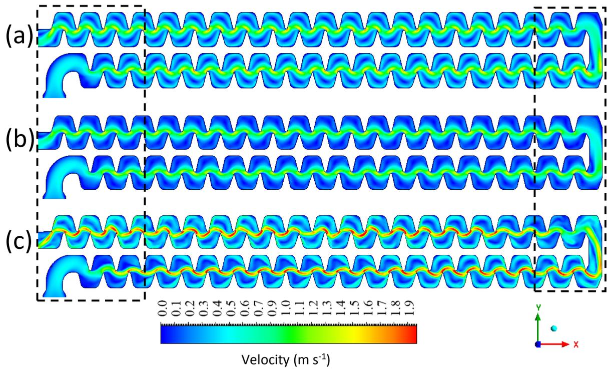
**Fig. 4.** Mean velocity fields obtained at  $z = 0.4$  mm using SKE (a), RSM (b), and LES (c) models. The velocity results were presented at the midpoint of the emitter's geometry at  $z = 0.4$  mm. The two black rectangles present the selected inlet and return zones to be studied in depth.
