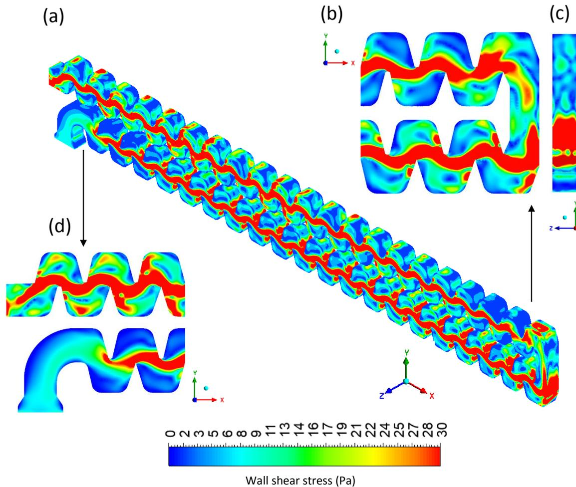
**Fig. 10.** Wall shear stress distribution along the flow path. (a) Three-dimensional representation of the labyrinth geometry highlighting the wall shear stress distribution. (b) Two-dimensional representation of the return zone within the  $(x,y)$  plane. (c) Two-dimensional representation of the return zone within the  $(y,z)$  plane. (d) Two-dimensional representation of the inlet zone within the  $(x,y)$  plane. The colour scale represents the magnitude of the wall shear stress in Pa.
