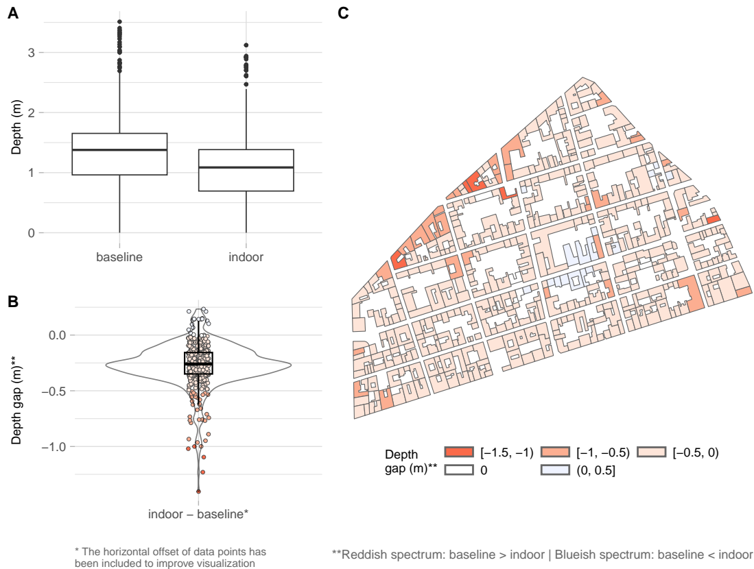
Figure 4: Differences in the estimated floodwater depth from the baseline scenario versus the indoor scenario: (A) comparison side by side of both scenarios; (B) density-boxplot of the differences between both scenarios; and (C) geographical distribution of the differences
