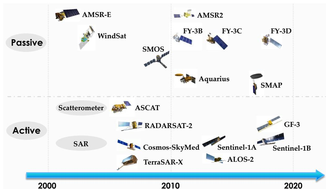
**Figure 1.** The primary microwave satellites/sensors that have been used to estimate soil moisture since the 2000. Note that both active and passive microwave sensors are mounted on the SMAP and Aquarius missions.
