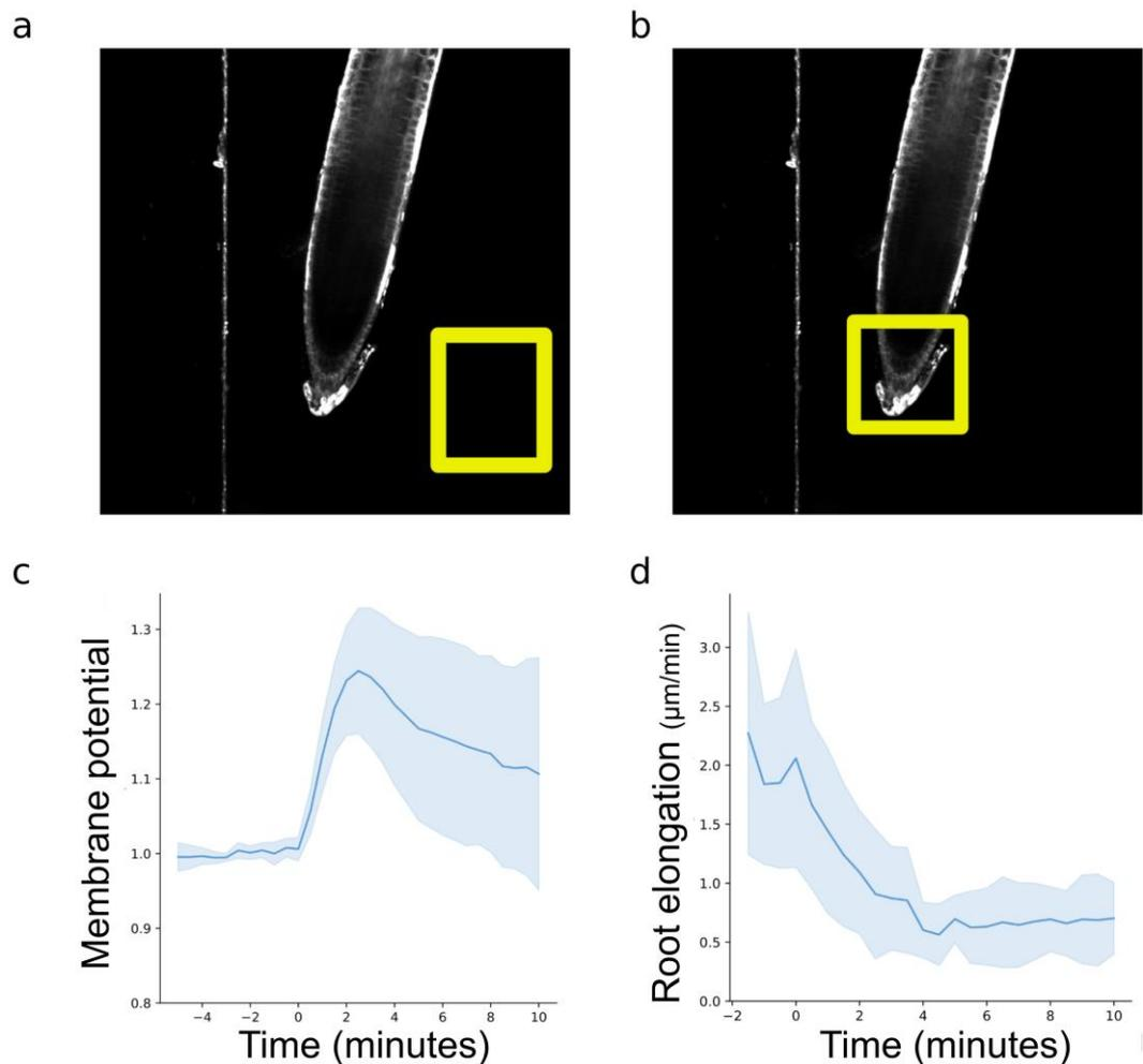
**Figure 4. Measurements and plotting microfluidic experiments.** (a) Selection of a background region of interest to determine the treatment arrival. (b) Rectangular selection of the root tip to determine root
