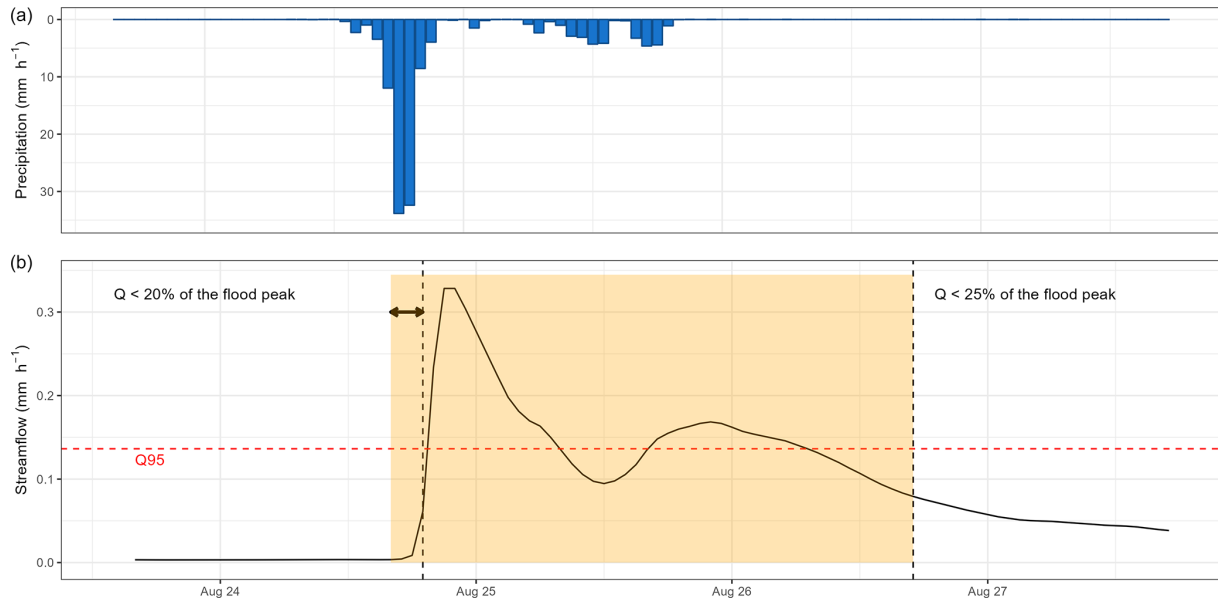
Figure A1. Flood event from 24 to 26 August 2009 on the Dore River at Saint-Gervais-sous-Meymont (K287191001). The yellow time window corresponds to the automatically selected event. The dashed red line represents the detection threshold set to the 95 % quantile. The dashed black lines refer to the initial entry and end dates of the events (respectively below 20 % and 25 % of the flood peak). The arrow here shows an extension of the event start due to the rapid rise in water level.
