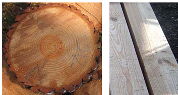
Fig. 6 Illustration of Pinus Pinaster Duramen characterised by a "darker red" colouring [1]
