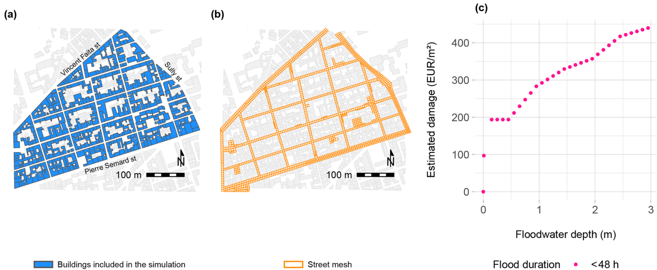
Figure 2. Experimental design: (a) buildings considered in the simulation perimeter; (b) street mesh in the simulation perimeter; (c) average national French damage function for short flood events (less than 48 h).
