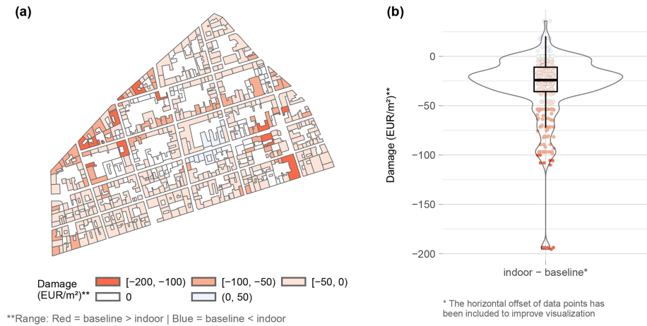
Figure 4. Differences in the estimates of damage per squared meter in the simulation perimeter between the baseline scenario and the indoor scenario: (a) geographical distribution; and (b) density-boxplot.
