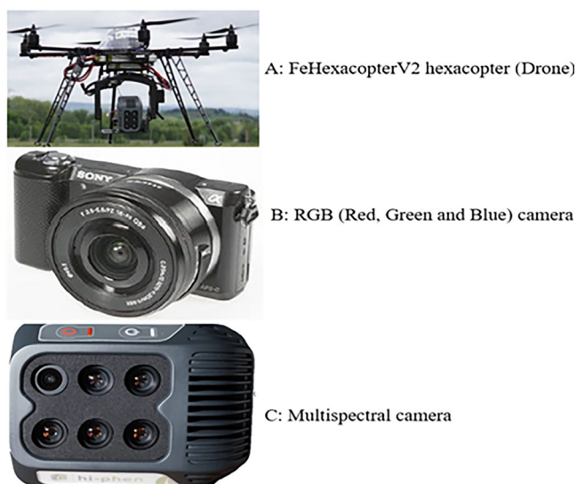
FIGURE 2 Drone (A), red, green, and blue (RGB) (B), and multispectral (C) cameras used in the image capture during the experiments in Senegal and Mali.
